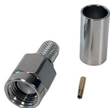
SMA (f) hun Product no: 17630 Type: Crimp Cable: RG58 Ohm: 50
