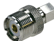
UHF (F) hun Product no: 40065 Type: Adapter Cable: FME Ohm: 50
